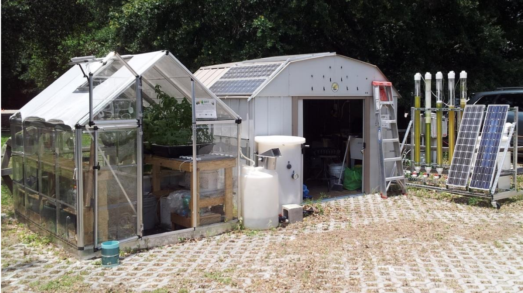
Figure 30 Pilot scale system incorporating small scale decentralized wastewater treatment with various resource recovery capabilities. Greenhouse hydroponics system and algae photobioreactors are located adjacent to a structure housing an AnMBR system.
